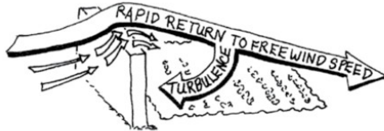
A solid barrier yields a sheltered area 8 times the height of the barrier but increases turbulence.
